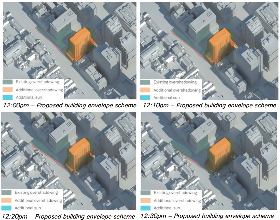
Figure 35 – Proposed building envelope and existing building shadow cast on RBA Building (14 April) Source: Hassell
