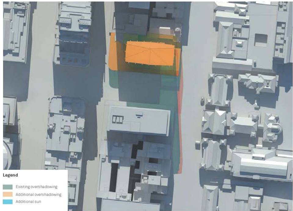
Figure 34 – Proposed building envelope and existing building shadow cast on 14 April at 12.00pm Source: Hassell
